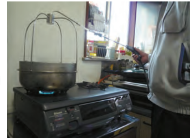
DME家庭用消費機器の燃焼性等の確認調査 Testing combustibility of home-use DME appliance
